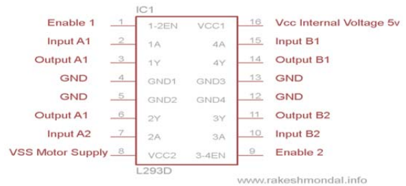
Fig. 7: Pin Configuration of Motor Driver
